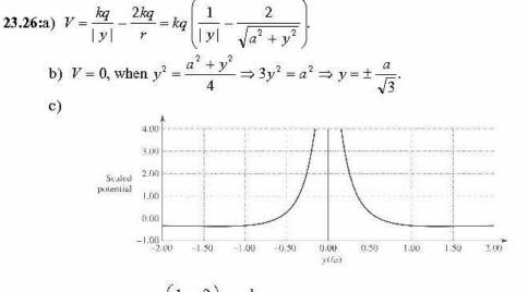
d)  $y >> a: V \approx kq \left(\frac{1}{y} - \frac{2}{y}\right) = -\frac{kq}{y}$ , which is the potential of a point charge -q.
